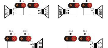
Two wire Bridge speakers to the Output sockets:
