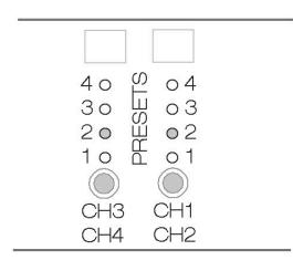
Located on the back panel of the DA2800-DSP/DA5000-DSP are two buttons labeled PRESET, each with four adjacent LED indicators. The layout is shown at left.
