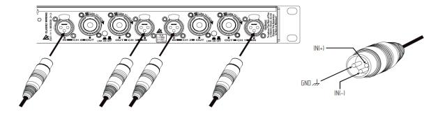
The figure below shows proper wiring for both balanced and unbalanced line inputs. Either type of configuration can be used, but we recommend using balanced connections because unbalanced cables (especially with long runs) can introduce noise into the audio system.
