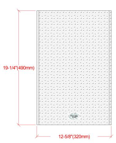
Wall cut-out =10.25"x17" (260x430mm) Weight = 6,5kg
